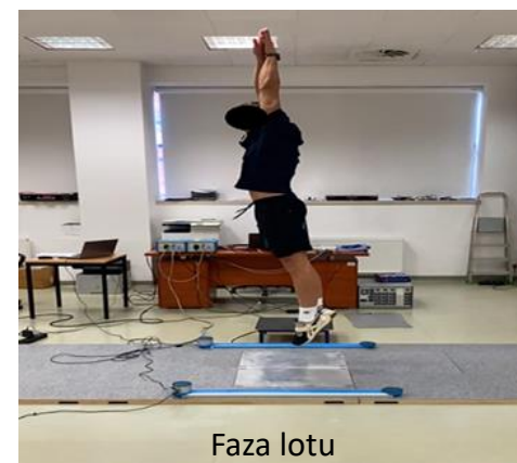
Ryc. 1. System Optogait i platforma Kistler
