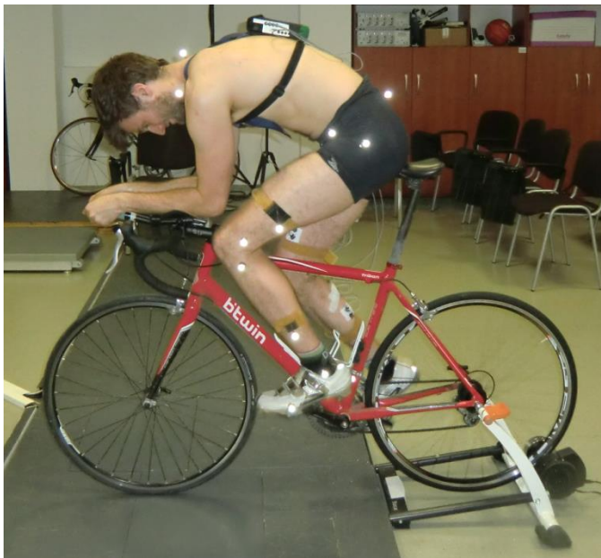
FIGURE 1. Measurement set-up. Bicycle with power measurement system is mounted in the rear hub and positioned on the cycle trainer. Telemetric EMG receiver is mounted on the subject's back.
